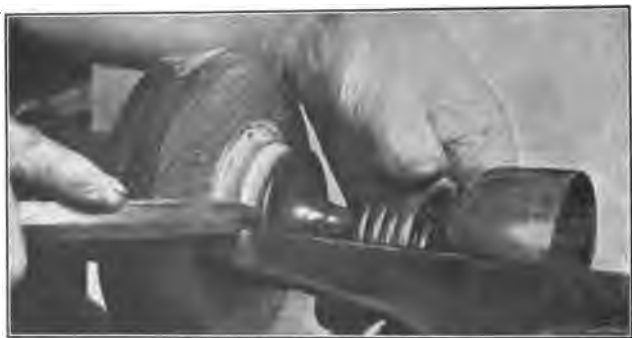
Fig. 122. Cutting Goblet from Chuck.
